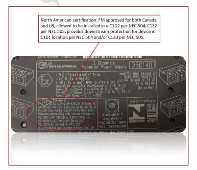
So to summarize here, the particular piece of equipment is certified for many different markets around the world by different third party labs, can be installed in Division 2/Zone 2 hazardous locations, can provide protection downstream of the area in which it is installed in an area of greater hazard such as Division 1 and/or Zone 0. Hopefully, this exercise has provided a little bit of clarification to help you understand Ex marking for a specific real world application.
