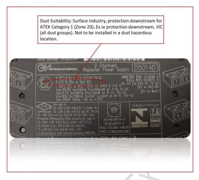
In this case, it can be used as an associated apparatus for providing protection downstream from the I.S. barrier into a Zone 20 dust location. However, unlike the gas application, this unit cannot be installed directly into a dust hazard location and must be located in a non-hazardous, ignitable dust free environment.
